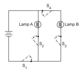
Which switch, when opened, causes both lamps to turn off?
