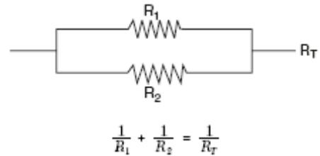
If  $R_1 = x$ ,  $R_2 = x + 3$ , and the total resistance,  $R_T$ , is 2.25 ohms, find the positive value of  $R_1$  to the *nearest tenth of an ohm*.
